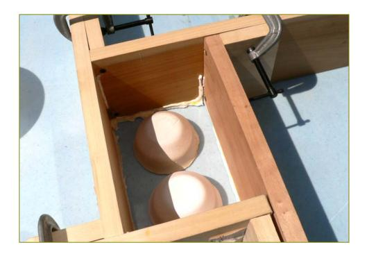
To create a simple mold box, we used several scrap pine boards, and a sheet of clear plexi-glass for the bottom.
